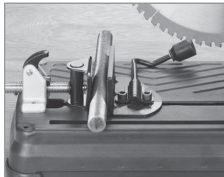
Cut forward of the blade center line and never cut bundles
