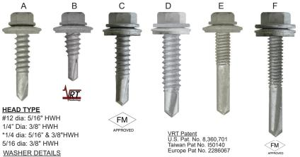
20 ga G-90 Galvanized Steel | Vulcanized to .062" thick non-conductive EPDM | 15MM OD Washer Special sizes available upon request
