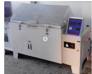
EXAMPLE OF KESTERNICH CABINET (ASTM G-85 SULFUR DIOXIDE TEST)
