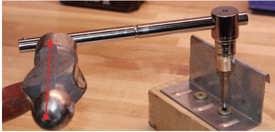
This is an example of how an impact tool works. It "hammers" the screw in a rotating fashion during installation.
